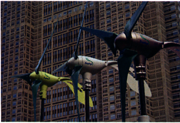
Fig. 4. New technology of carbon-reinforced material in small wind turbine of Airdolphin by Zepher
